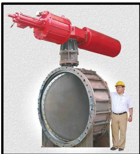
72" Pneumatic operated (ESD) For Bhushan Closing time < 3 sec
